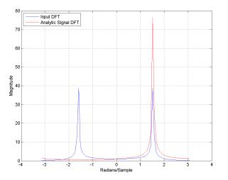
Design a minimum-order Hilbert transformer that has a sampling frequency of 1 kHz. Specify the passband ripple to be 1 dB.
