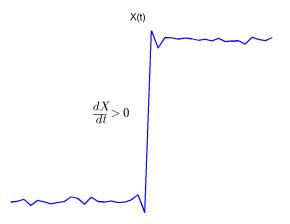
In the preceding figure, the amplitude values of the waveform do not appear because a positive-going transition does not depend on the actual waveform values. A positive-going transition is defined by the direction of the transition.
