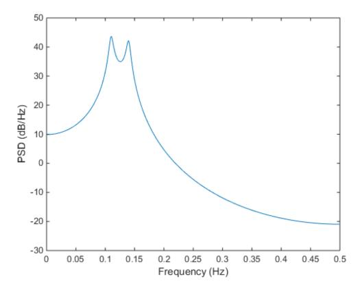
Create a realization of the AR(4) random process. Set the random number generator to the default settings for reproducible results. The realization is 1000 samples in length. Assume a sampling frequency of 1 Hz. Use pyulear to estimate the PSD for a 4th-order process. Compare the PSD estimate with the true PSD.
