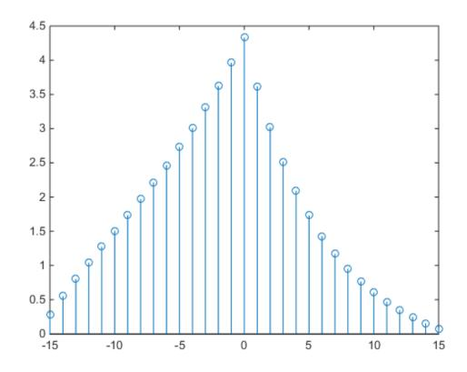
Determine *c* analytically to check the correctness of the result. Use a larger sample rate to simulate a continuous situation. The cross-correlation function of the sequences  $x_a(n) = a^n$  and  $x_b(n) = b^n$  for  $n \ge 0$ , with 0 < a, b < 1, is
