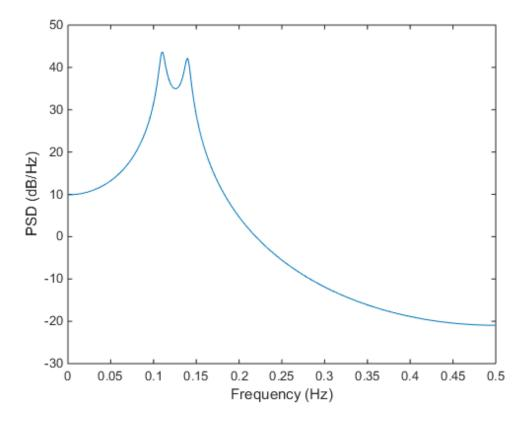
Create a realization of the AR(4) random process. Set the random number generator to the default settings for reproducible results. The realization is 1000 samples in length. Assume a sampling frequency of 1 Hz. Use pburg to estimate the PSD for a 4th-order process. Compare the PSD estimate with the true PSD.
