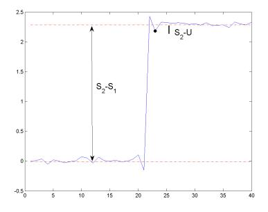
The red dashed lines indicate the estimated state levels. The double-sided black arrow depicts the difference between the high- and low-state levels. The solid black line indicates the difference between the high-state level and the undershoot value.
