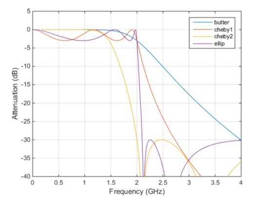
The Butterworth and Chebyshev Type II filters have flat passbands and wide transition bands. The Chebyshev Type I and elliptic filters roll off faster but have passband ripple. The frequency input to the Chebyshev Type II design function sets the beginning of the stopband rather than the end of the passband.
