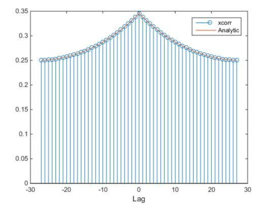
Repeat the calculation, but now find a *biased* estimate of the autocorrelation. Verify that the biased estimate is given by  $c_b(n) = c(n)/N$ .
