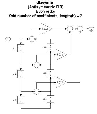
Note that antisymmetry is defined as b(i) == -b(end - i + 1) so that the middle coefficient is zero for odd length b((end+1)/2) = 0
