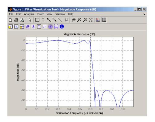
Display and analyze multiple FIR filters, starting FVTool from the command line. Then, display the associated analysis parameters for the magnitude:
