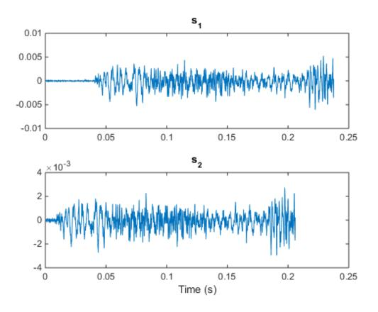
The cross-correlation of the two measurements is maximum at a lag equal to the delay.
