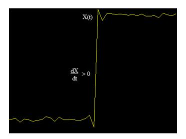
Whenever there is a plus sign (+) next to a text label, this symbol refers to measurement associated with a rising edge, a transition from a low-state level to a high-state level.
