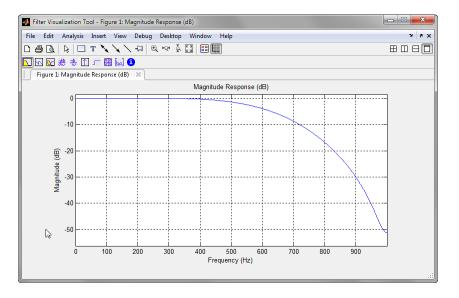
The cutoff does not look particularly sharp. The response is above 40 dB for most frequencies. You remember that the assistant had an option to set up a "magnitude constraint" called the "stopband attenuation". Open the assistant by calling designfilt with the filter name as input.
