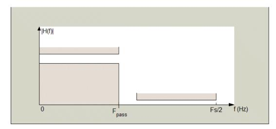
In the figure, the transition region lies between the end of the passband and the start of the stopband. The width is defined explicitly by the value of **Transition width**.
