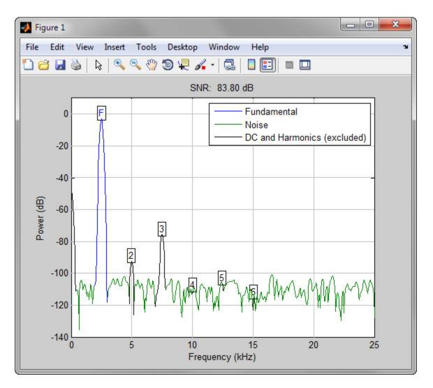
The DC component and all harmonics, including the fundamental, are excluded from the noise measurement. The fundamental and harmonics are labeled.
