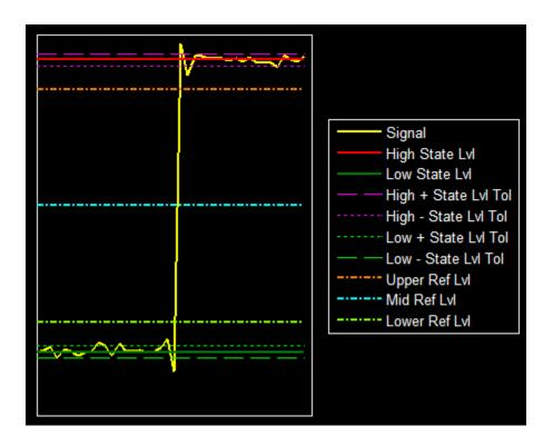
the high-state level, low-state level, state-level tolerance, upper-reference level, midreference level, and lower-reference level, as shown in the following figure.
