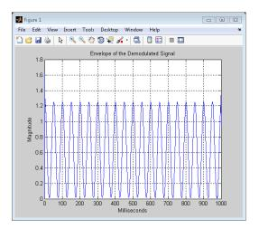
From the preceding figure, you see that the envelope completes two cycles every 100 milliseconds. The envelope is oscillating at 20 Hz, which corresponds to the frequency of the message signal.
