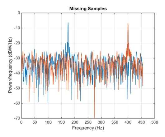
Sample the original signal, but make the sampling nonuniform by adding jitter (uncertainty) to the time measurements. The first instant continues to be at zero. Use plomb to estimate and plot the PSD of the nonuniformly sampled signal.
