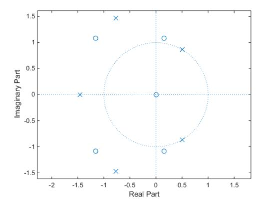
bb and aa are equivalent to b and a, respectively. However, the system is unstable because it has poles outside the unit circle. Use invfreqz's iterative algorithm to find a stable approximation to the system. Verify that the poles are within the unit circle.
