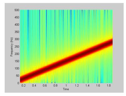
Compute the spectrogram of a chirp with quadratic instantaneous frequency deviation:
