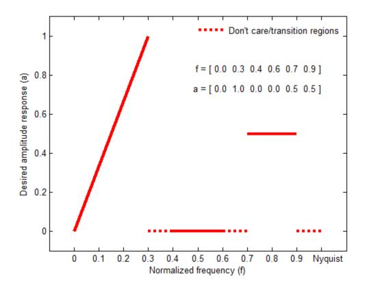
b = firls(n, f, a, w) uses the weights in vector w to weight the fit in each frequency band. The length of w is half the length of f and a, so there is exactly one weight per band.
