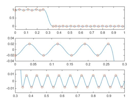
The Bound Violations denote the iterations of the procedure as the design converges. Display the magnitude response of the filter.
