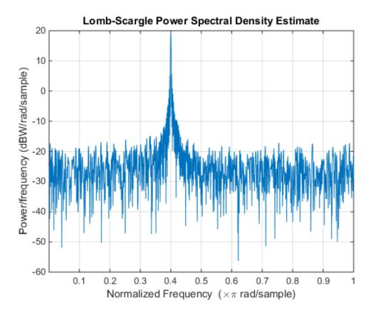
Remove every other sample by assigning NaN's. Use plomb to compute and plot the PSD. The periodogram peaks at the same frequency because the time axis is unchanged.
