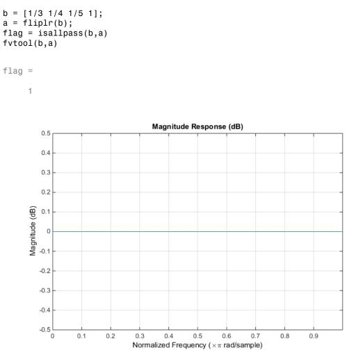
Create a lattice allpass filter and verify that the filter is allpass.
