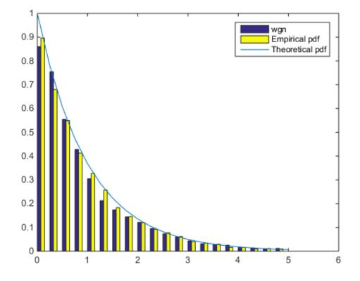
Embed in the noise a sinusoidal signal of frequency 0.1 Hz. Use a signal-to-noise ratio of  $\xi = 0.01$ . Specify the sinusoid amplitude,  $x_0$ , using the relation  $x_0 = \sigma \sqrt{2\xi}$ . Compute the power spectrum of the signal and plot its histogram alongside the empirical and theoretical distribution functions.
