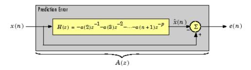
Input vector **a** represents the polynomial coefficients of this prediction error filter in descending powers of z.
