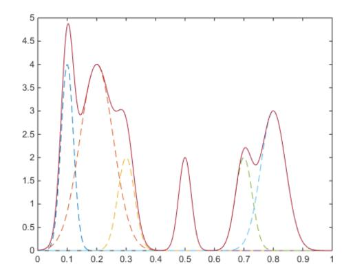
Measure the widths of the peaks using the half prominence as reference.
