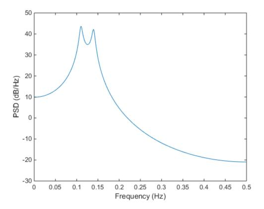
Create a realization of the AR(4) random process. Set the random number generator to the default settings for reproducible results. The realization is 1000 samples in length. Assume a sampling frequency of 1 Hz. Use pcov to estimate the PSD for a 4th-order process. Compare the PSD estimate with the true PSD.
