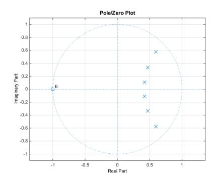
Given a filter defined with a set of single-precision numerator and denominator coefficients, check if it has minimum phase for different tolerance values.
