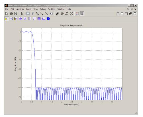
The next example designs a lowpass equiripple filter with a direct-form transposed structure and density factor of 20 by specifying the FilterStructure and DensityFactor properties.
