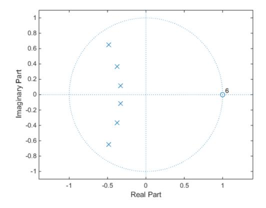
Redesign the filter using designfilt and check it for stability.
