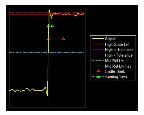
You can modify the settle seek duration parameter in the **Settings** pane. For more information on the algorithm this measurement uses, see the Signal Processing Toolbox settlingtime function reference.
