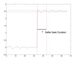
**settlingtime** may fail to find a settling point in the specified settle seek duration if any one of the following conditions occurs:
