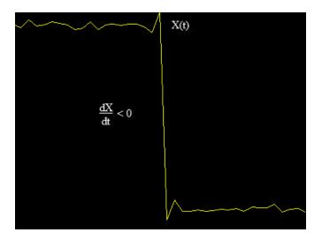
Whenever there is a minus sign (–) next to a text label, this symbol refers to measurement associated with a falling edge, a transition from a high-state level to a low-state level.
