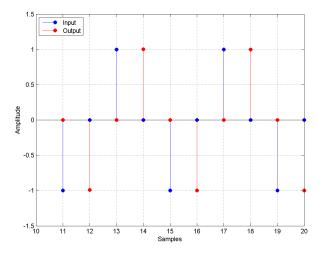
Because the frequency of the discrete-time sinusoid is  $\pi/2$  radians/sample, a one sample shift corresponds to a phase shift of  $\pi/2$ .
