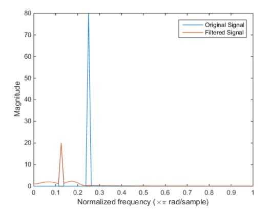
Create a filter of order 10 with a 6-dB frequency of 9.6 kHz and a sampling frequency of 48 kHz. The only valid design method is the FIR window method.
