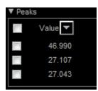
The numerical values displayed in the **Value** column are equivalent to the **pks** output argument returned when you run the findpeaks function. The numerical values displayed in the second column are similar to the **locs** output argument returned when you run the findpeaks function.
