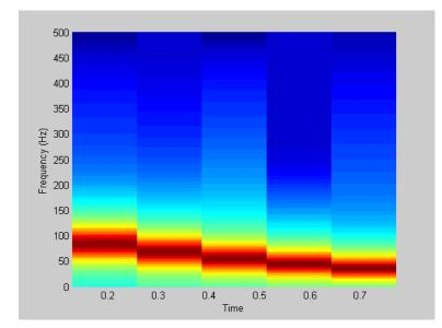
Compute the spectrogram of a logarithmic chirp:
