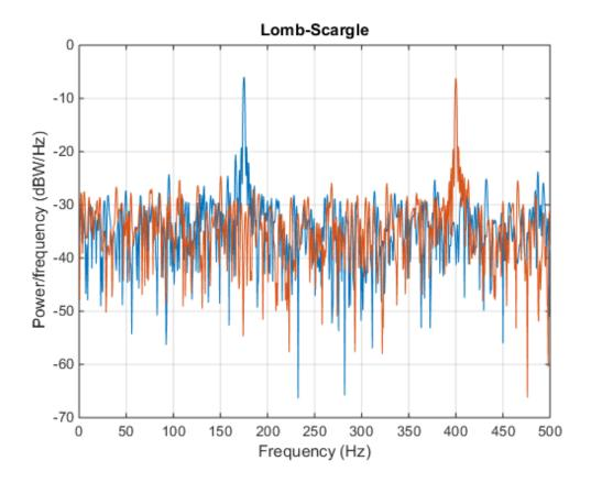
Suppose the signal is missing 10% of the original samples. Place NaN's in random locations to simulate the missing data points. Use plomb to estimate and plot the PSD of the signal with missing samples.
