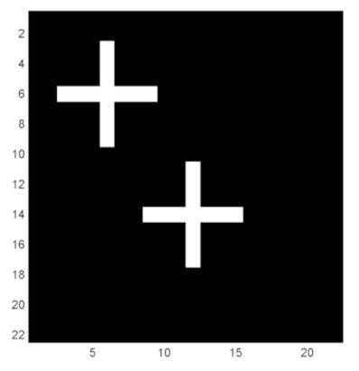
Cross-correlate the two matrices and find the maximum absolute value of the crosscorrelation. Use the position of the maximum absolute value to determine the shift in the template. Check the result against the known shift.
