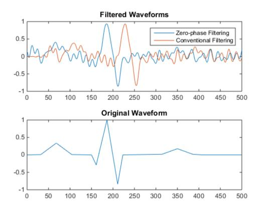
Zero-phase filtering reduces noise in the signal and preserves the QRS complex at the same time it occurs in the original. Conventional filtering reduces noise in the signal, but delays the QRS complex.
