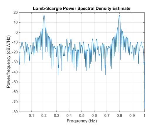
The aliasing results from the fact that the frequency of the sinusoid is greater than the Nyquist frequency.
