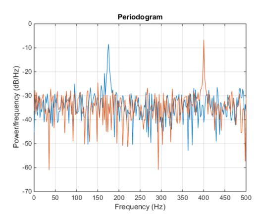
Use plomb with the default settings to estimate and plot the PSD of the signal. Use the axis limits from the previous plot.
