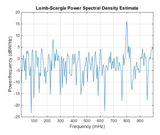
The aliasing disappears. The irregular sampling increases the effective sample rate by shrinking some time intervals.
