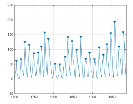
Use the peak locations returned by findpeaks to compute the mean interval between maxima.
