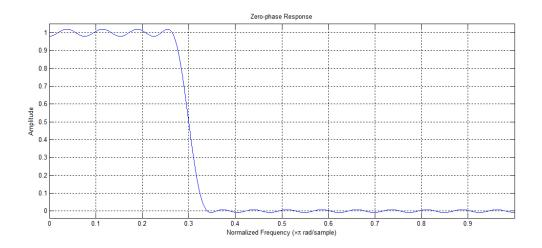
Design the same filter using fircls1. Keep in mind that fircls1 uses linear units to measure the ripple and attenuation. Display the zero-phase response.
