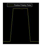
Equivalently, a positive-polarity (positive-going) pulse has a terminating state more positive than the originating state.
