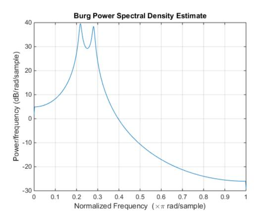
Burg PSD Estimate of a Multichannel Signal
