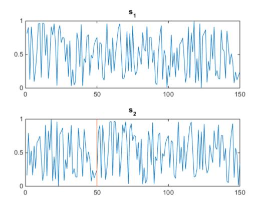
Compute biased estimates of the autocovariance and mutual cross-covariance sequences. The output array is organized as  $\mathbf{c} = (c_{s_1s_1} \quad c_{s_1s_2} \quad c_{s_2s_1} \quad c_{s_2s_2})$ . Plot the result. The maxima at  $\mp 50$  and  $\pm 100$  are a result of the circular shift.
