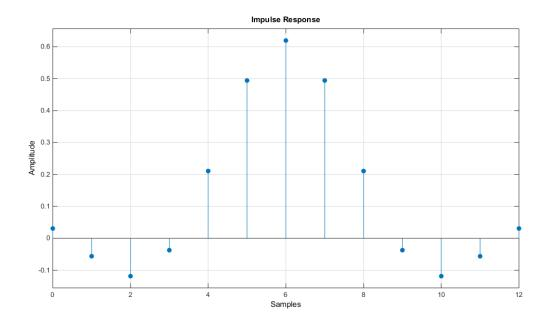
Convolve the square-root filter with itself. Truncate the impulse response outward from the maximum so it has the same length as h1. Normalize the response using the maximum. Then, compare the convolved square-root filter to the normal filter.
