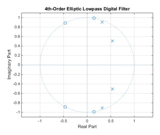
Create the same filter using designfilt. Use fvtool to plot its poles and zeros.
