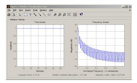
Generate length N=128 rectangular window, return values, and write ASCII file: H=sigwin.rectwin(128);
