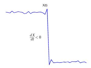
In the preceding figure, the amplitude values of the waveform are not displayed because a negative-going transition does not depend on the actual waveform values. A negativegoing transition is defined by the direction of the transition.
