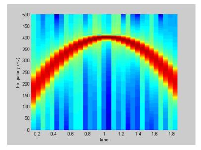
Compute the spectrogram of a concave quadratic chirp:
