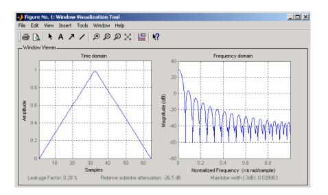
Create a 128-point Chebyshev window with 100 dB of sidelobe attenuation. (See chebwin for information on Chebyshev windows.) View the results of this and the above Bartlett window in the Window Design and Analysis Tool (wintool):
