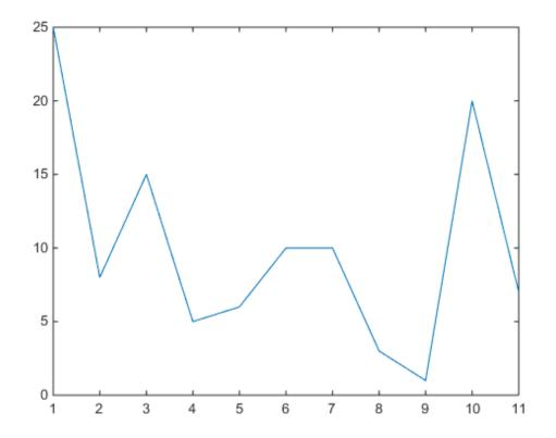
Find the local maxima. The peaks are output in order of occurrence. The first sample is not included despite being the maximum. For the flat peak, the function returns only the point with lowest index.
