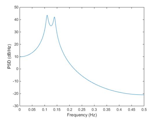
Create a realization of the AR(4) random process. Set the random number generator to the default settings for reproducible results. The realization is 1000 samples in length. Assume a sampling frequency of 1 Hz. Use pmcov to estimate the PSD for a 4th-order process. Compare the PSD estimate with the true PSD.
