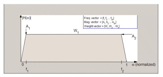
In the figure, the regions between 0 and  $f_1$  and between  $f_2$  and 1 represent the transition regions where the filter response is explicitly defined by the transition width.
