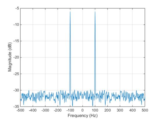
You see that the power at -100 and 100 Hz is close to the expected power of 1/4 for a real-valued sine wave with an amplitude of 1. The deviation from 1/4 is due to the effect of the additive noise.
