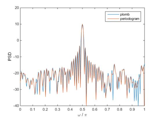
Estimate the Lomb-Scargle PSD of a three-channel signal composed of sinusoids. Specify the frequencies as  $2\pi/3$  rad/sample,  $\pi/2$  rad/sample, and  $2\pi/5$  rad/sample. Add white Gaussian noise of variance 1/100. Use plomb with no output arguments to compute and plot the PSD estimate in decibels.
