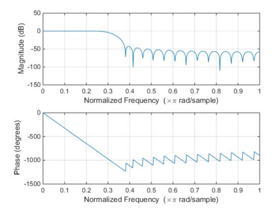
Design an odd-length bandpass filter. Note that odd length means even order, so the input to fir1 must be an even integer.
