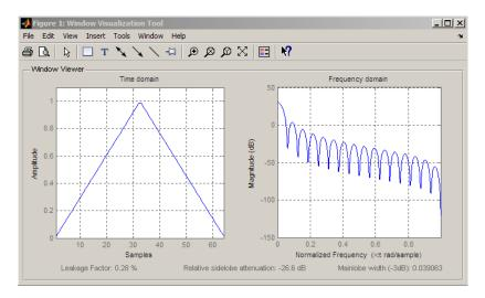
Generate length L = 128 triangular window, return values, and write ASCII file:
