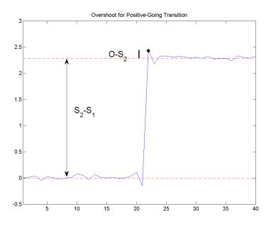
The red dashed lines indicate the estimated state levels. The double-sided black arrow depicts the difference between the high and low-state levels. The solid black line indicates the difference between the overshoot value and the high-state level.
