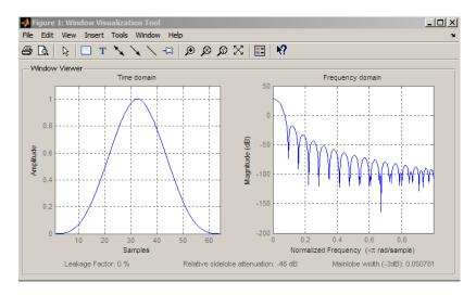
Generate length N=128 Bohman window, return values, and write ASCII file:
