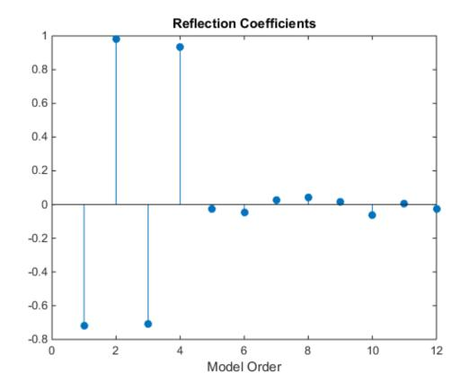
The reflection coefficients decay to zero after order 4. This indicates an AR(4) model is most appropriate.
