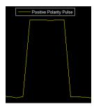
Equivalently, a positive-polarity (positive-going) pulse has a terminating state more positive than the originating state.
