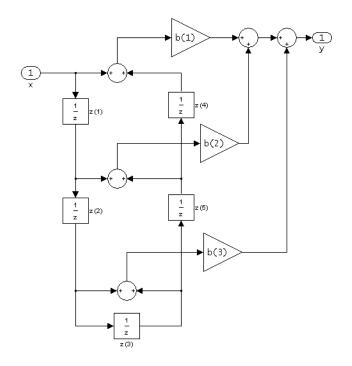
The resulting filter states column vector for the odd number of coefficients example above is
