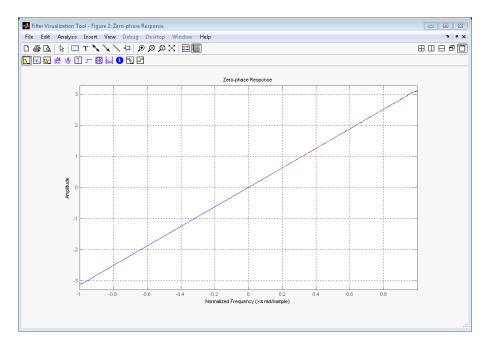
Design a narrow band differentiator. Differentiate the first 25 percent of the frequencies in the Nyquist range and filter the higher frequencies.
