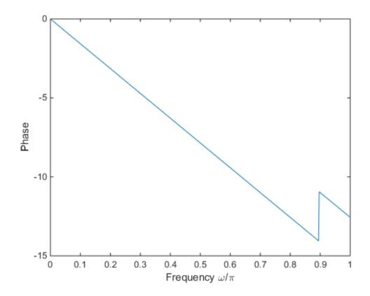
IIR filters in general do not have linear phase. Verify the statement by constructing eighth-order Butterworth, Chebyshev, and elliptic filters with similar specifications.
