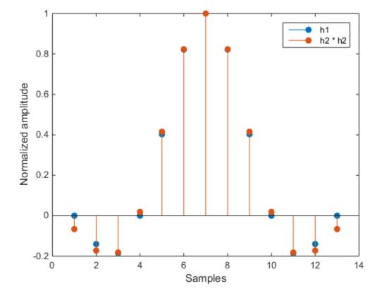
The convolved response does not coincide with the normal filter because of its finite length. Increase **span** to obtain closer agreement between the responses and better compliance with the Nyquist criterion.
