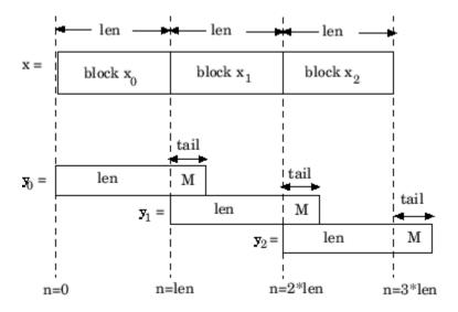
where len is the block length and M is the length of the numerator-1, (length(b)-1), which is also the number of states. The output of each convolution is a block that is longer than the input block by a tail of (length(b)-1) samples. These tails overlap the next block and are added to it. The states reported by dfilt.fftfir are the tails of the final convolution.
