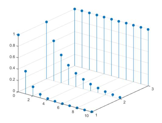
Compute the autocorrelations and mutual cross-correlations of the sequences. Output the lags so you do not have to keep track of them. Normalize the result so the autocorrelations have unit value at zero lag.
