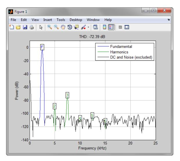
The plot shows the spectrum used to compute the ratio and the region treated as noise. The DC level is excluded from the computation. The fundamental and harmonics are labeled.
