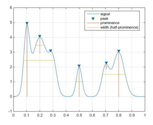
Measure the widths again, this time using the half height as reference.
