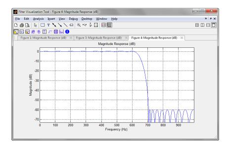
A little experimentation shows that you can obtain a similar filter by setting the passband and stopband frequencies respectively to 600 Hz and 700 Hz.
