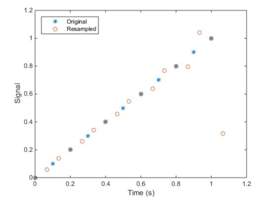
Notice that the last few points of the output, y, are inaccurate. In its filtering process, resample assumes that the input sequence, x, is zero before and after the samples it is given. Thus, large deviations from zero at the endpoints of x can cause inaccuracies in y at its endpoints. The following two plots illustrate this side effect of resample.
