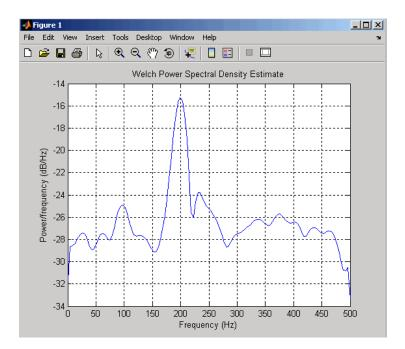
The following example produces a result similar to the obsoleted **spectrum** function, which used a Hann window as the default.
