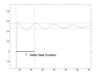
In the preceding figure, you see that the last sample in the settle seek interval exceeds the upper state boundary. In this example, reducing or increasing the settle seek duration can result in a valid settling time.
