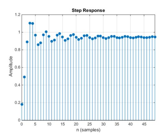
Create the same filter using designfilt and display its step response using fvtool.
