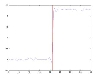
The instant at which the waveform crosses the 50% reference level is 21.5. Note that this is not a sampling instant present in the input vector because midcross uses interpolation to identify the mid-reference level crossing.
