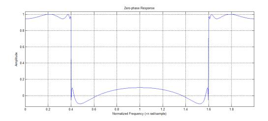
Create the same filter using ellip. Plot its zero-phase response.
