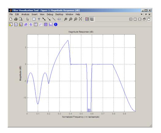
Now design the arbitrary-magnitude complex FIR filter. Recall that vector f contains frequency locations and vector a contains the desired filter response values at the locations specified in f.
