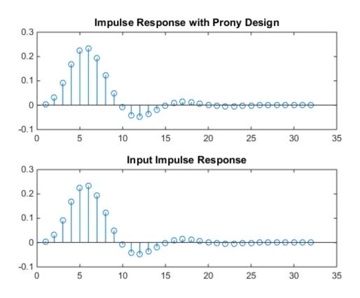
Fit a 10th-order FIR model to the impulse response of a highpass filter. Plot the original and Prony-designed frequency responses.
