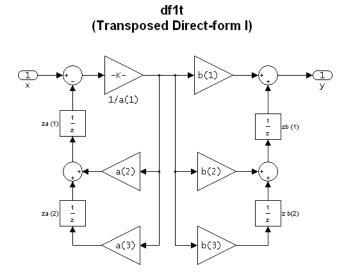
To display the filter states, use this code to access the filtstates object.
