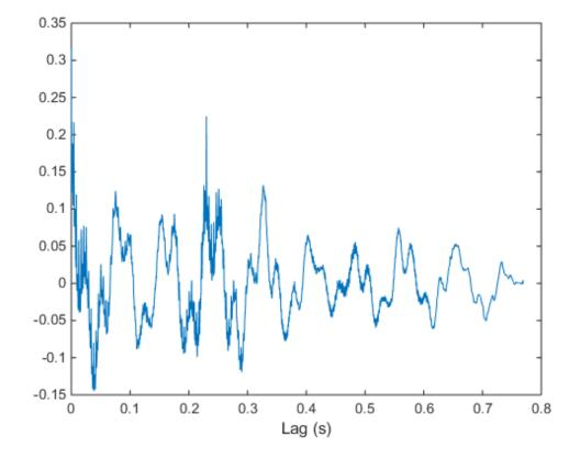
The autocorrelation has a sharp peak at the lag at which the echo arrives. Cancel the echo by filtering the signal through an IIR system whose output, w, obeys  $w(n) + \alpha w(n - \Delta) = y(n)$
