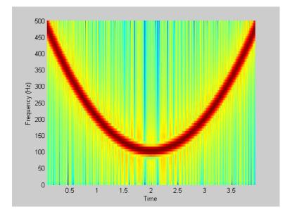
Compute the spectrogram of a convex quadratic chirp:
