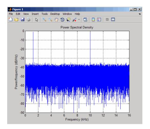
% Create a double-sided spectrum Hpsd = dspdata.psd(Pxx,'Fs',Fs,'SpectrumType','twosided'); plot(Hpsd)
