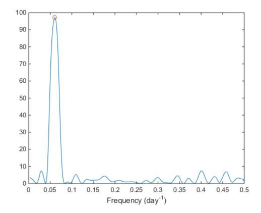
Determine Callisto's orbital period (in days) as the inverse of the frequency of maximum energy. The result differs by less than 1% from the value published by NASA.
