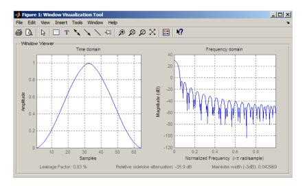
Generate length N=128 modified Bartlett-Hanning window, return values, and write ASCII file with window values:
