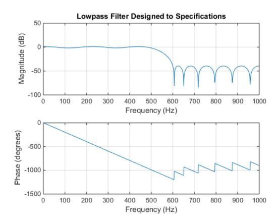
Note that the filter falls slightly short of meeting the stopband attenuation and passband ripple specifications. Using n+1 in the call to firpm instead of n achieves the desired amplitude characteristics.
