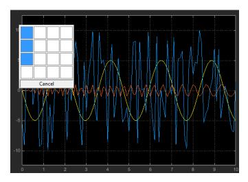
After you select row 3, column 1, the scope window is partitioned into three separate displays, as shown in the following figure.
