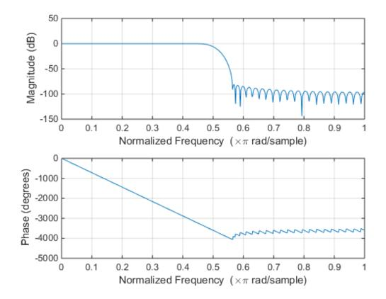
Design the same filter using designfilt. Display its magnitude and phase responses using fvtool.
