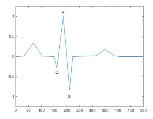
The QRS complex is an important feature in the ECG. Here it begins around time point 160.
