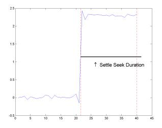
• An intervening transition is detected before the end of the specified settle seek duration. The following figure illustrates this condition for a settle seek duration of 22 samples. An intervening transition is detected before the end of the 22–sample settle seek duration.
