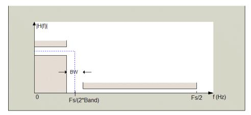
In the figure, BW is the width of the transition region and **Band** determines the location of the center of the region.
