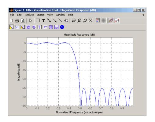
Create an elliptic filter and use some of FVTool's figure handle commands:
