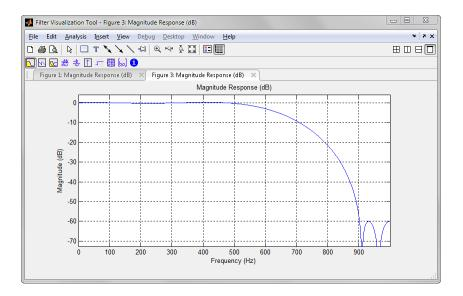
The cutoff still does not look sharp. The attenuation is indeed 60 dB, but for frequencies above 900 Hz.
