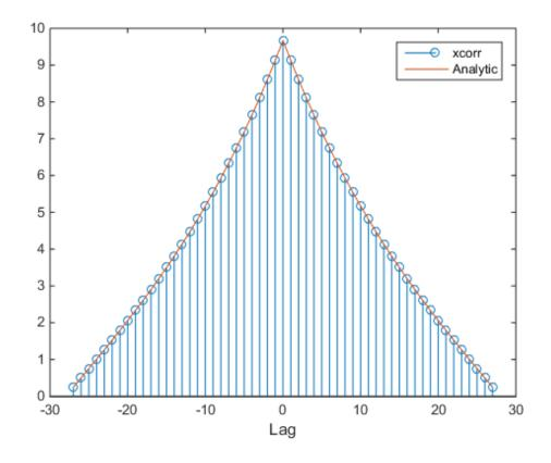
Repeat the calculation, but now find an *unbiased* estimate of the autocorrelation. Verify that the unbiased estimate is given by  $c_u(n) = c(n)/(N - |n|)$ .
