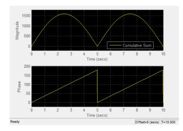
This feature is particularly useful for complex-valued input signals. If the input is a realvalued signal, selecting this check box returns the absolute value of the signal for the magnitude. The phase is 0 degrees for nonnegative input and 180 degrees for negative input.
