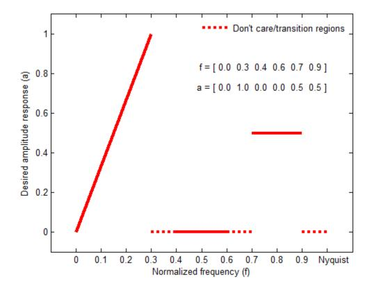
firpm always uses an even filter order for configurations with even symmetry and a nonzero passband at the Nyquist frequency. This is because for impulse responses exhibiting even symmetry and odd orders, the frequency response at the Nyquist frequency is necessarily 0. If you specify an odd-valued n, firpm increments it by 1.
